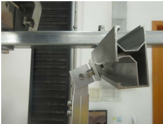
Photo 5: part view after destruction
